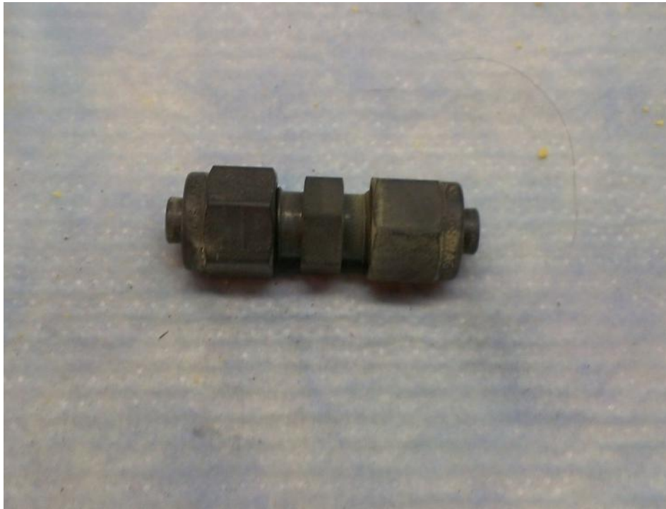
Figure 4.23. Sealed Swagelok Volume after Heating in Tube Furnace
