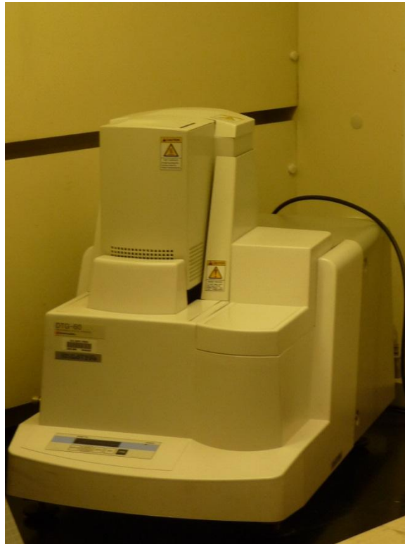
Figure 3.1. Installation of DTG-60
