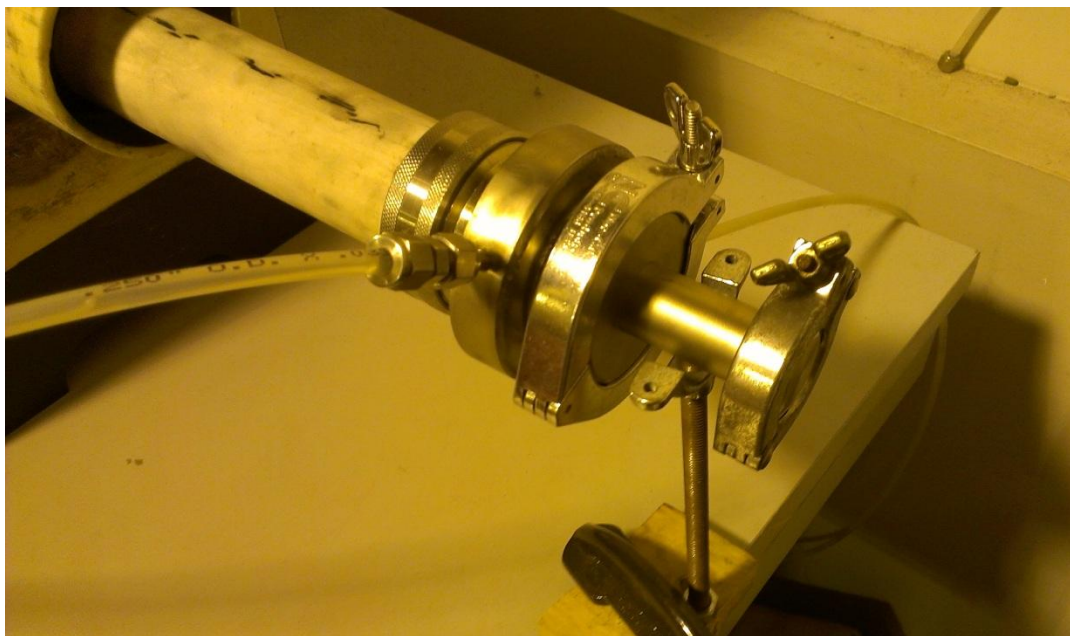
Figure 3.9. Close-up of Cooling Water Jacket and End Caps
